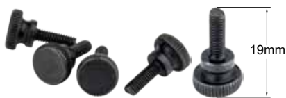
KS-292 M4 Knurled Shoulder Steel Thumb Screw Knurled head type screws, ideal for VESA mount monitor, have a pattern of ridges that allow for easy gripping and tightening by hand. The threaded shaft is 12mm in length and total length including the shoulder and head is 19mm. (Set of 4)
