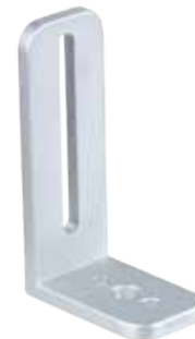
KS-2439C Mini L-Cheese Plate w/ Camera Bracket W 30g / 1.05oz L-Cheese plate measures 2.4" (6cm) x 1.37" (3.5cm) on the long leg with camera bracket and 3.9" (10cm) x 1.37" (3.5cm) on the small leg with 3/8" & 1/4" holes. Thickness: 0.236" (6mm)
