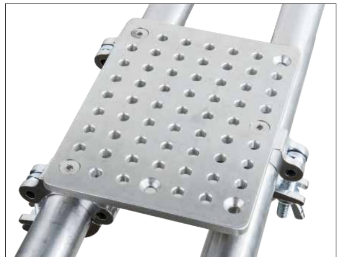
KCP-830CP Coupler for Cheese Plate W 0.52kg / 1.2lb Slim type half coupler for tube dia.2" (48~51mm) with a 3/8"-16 threaded female & stainless steel bolt.
