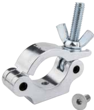
KCP-830CP Coupler for Cheese Plate W 0.52kg / 1.2lb Slim type half coupler for tube dia.2" (48~51mm) with a 3/8"-16 threaded female & stainless steel bolt.
