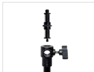
A steel made universal adaptor spigot in black featuring a double-sided baby 5/8" (16mm) stud with 1/4"-20 male thread on one side and a 3/8"-16 male thread on the other
