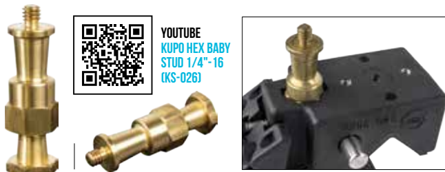
KS-026 Hex Baby Stud 1/4"-20 W 70g 2.47oz Solid brass made, this stud comes with hex end for Convi Clamp and the other round end for lighting fixture. It also allows rotating while connecting two Convi clamps. 5/8" (16mm) baby stud with 1/4"-20 male threads.
