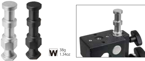
KS-020 / KS-020B 5/8" Compact Alu. Snap in Pin W 38g 1.34oz Lightweight aluminum 5/8" (16mm) adapter with hex stud for Convi clamp and round head in the other side. Special for Desisti & laniro lighting fixtures.
