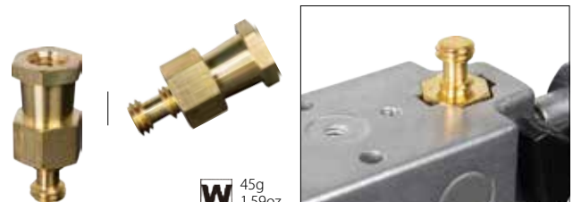
KS-038 Hex Adapter w/ 3/8"-16F & 3/8"-16M W 45g 1.59oz Solid brass made 5/8" hex adapter keeps it from rotating in Convi clamp with one end 3/8"-16 female threads and the other end 3/8"-16 male threads.
