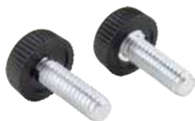
KS-292 M4 Knurled Shoulder Steel Thumb Screw Knurled head type screws, ideal for VESA mount monitor, have a pattern of ridges that allow for easy gripping and tightening by hand. The threaded shaft is 12mm in length and total length including the shoulder and head is 19mm. (Set of 4)
