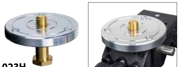
KS-023H 3/8"-16 Head Mounting Plate w/ Hex Stud W 100g 3.53oz Round flat plate made to mount ball head or any other accessory tapped with a 3/8"-16 threads for Convi clamp. Features a hex stud which keeps the stud from rotating inside the Convi clamp.
